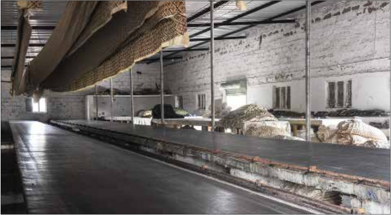
A workshop for screen printing ajrakh , Dhamadka, Kutch. Originally, Khatri hand printed squatting at small tables low to the ground, then standing at higher 6 meter tables. The demands for cheap printed fabric in quantity have led to industrial innovations such as screen instead of hand printing, on tables as long as 40 meters. Photo credit: Judy Frater 2019.
